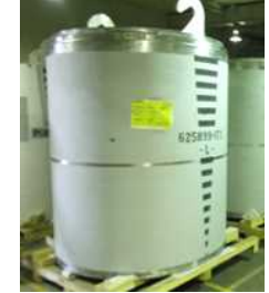
HIC※1 (after attaching stainless reinforcement body)
