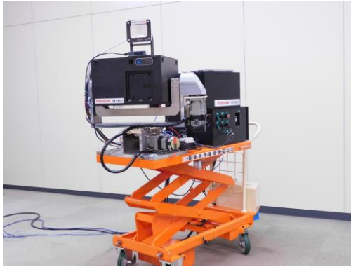
Contamination measurement by using \alpha camera
