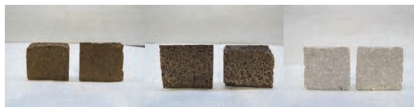
Figure 2 Sludge and slurry waste streams cross section observation
