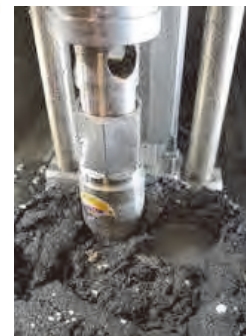
Core boring on a block of ex-vessel fuel debris simulant
